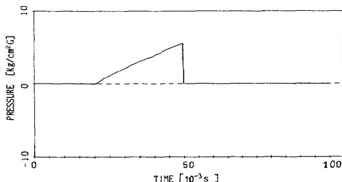
Fig. 7. Example of pressure rate pattern by N<sub>2</sub> method (Dutch pressure vessel, 0.1 mm<sup>t</sup> Al rupture disk, sampling time 100 ms,  $P_{\max}$  5.6 kg/cm<sup>2</sup>,  $(dP/dt)_{\max}$  = 0.17 kg/cm<sup>2</sup>/s).
