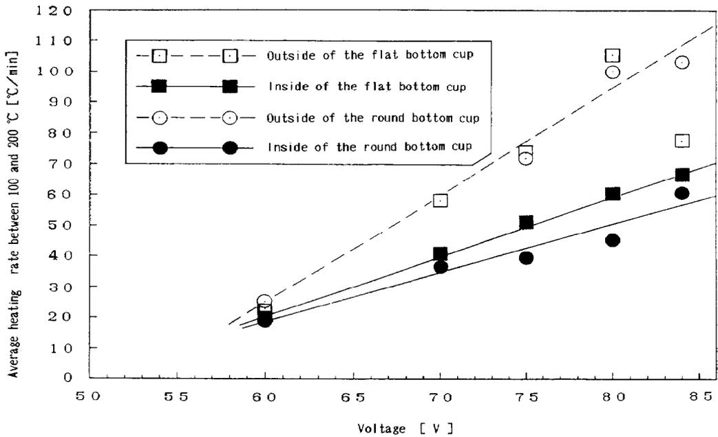
Fig. 6. Heating rate characteristic of US pressure vessel.
