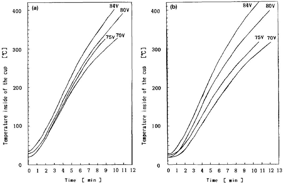
Fig. 3. Heating rate curves of Dutch pressure vessel: (a) flat bottom cup, and (b) round bottom cup. Voltage was varied to 70, 75, 80 and 84 V, respectively.
