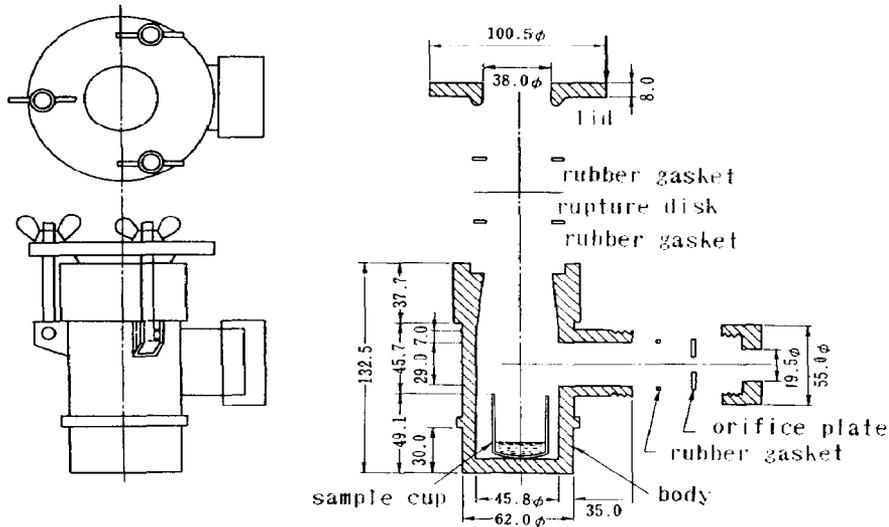
Fig. 2. Schematic of US pressure vessel.
