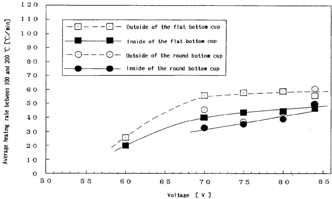
Fig. 5. Heating rate characteristic of Dutch pressure vessel.
