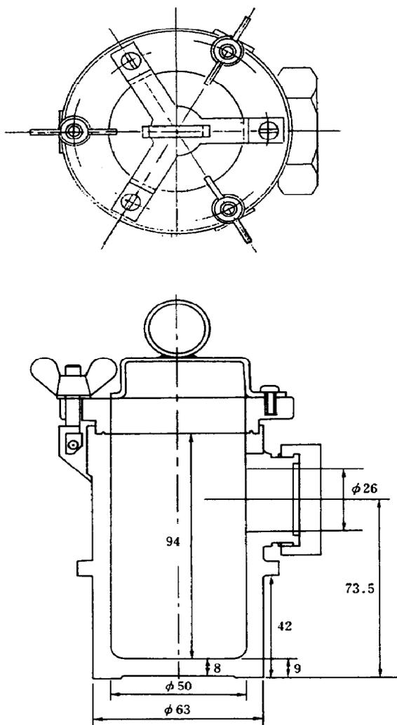
Fig. 1. Schematic of Dutch pressure vessel.
