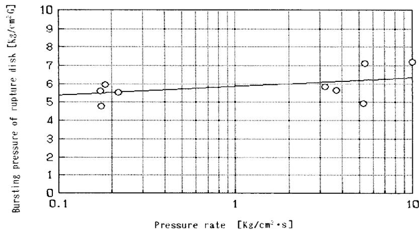
Fig. 8. Relationship between bursting pressure and N<sub>2</sub> pressure rate (Dutch vessel, 0.1 mm<sup>t</sup> Al rupture disk).
