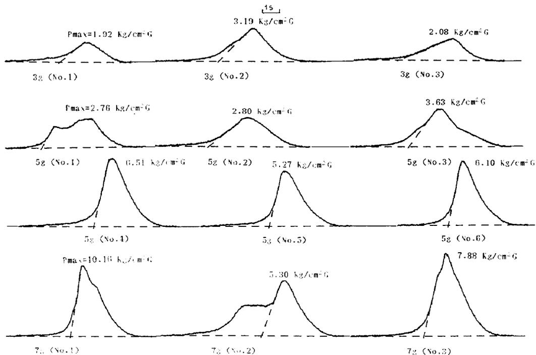
Fig. 12. Examples of pressure pattern of the decomposition reaction of ADCA. (Dutch vessel, flat bottom cup, ADCA mass 3–7 g, 70 V, 1 mm orifice).
