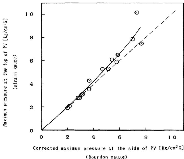
Fig. 11. Relationship between maximum pressure of strain gauge measured at the top of the pressure vessel and the corrected maximum pressure measured by the Bourdon gauge at the vessel side. (Dutch vessel, flat bottom cup, ADCA mass 3-7 g, voltage of electric furnace 70 V, 1 mm diameter orifice.)
