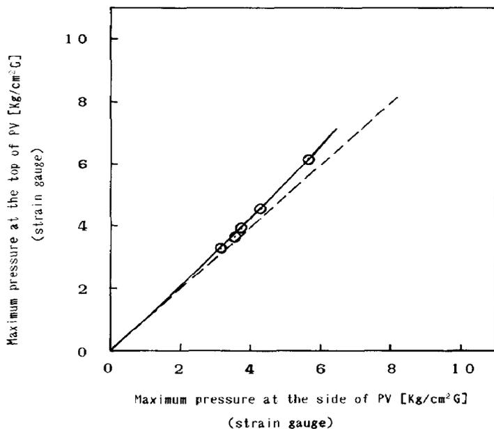
Fig. 13. Relationship between the maximum pressure measured by strain gauges at the top and the side of the pressure vessel. (Vessel details, see Fig. 12).
