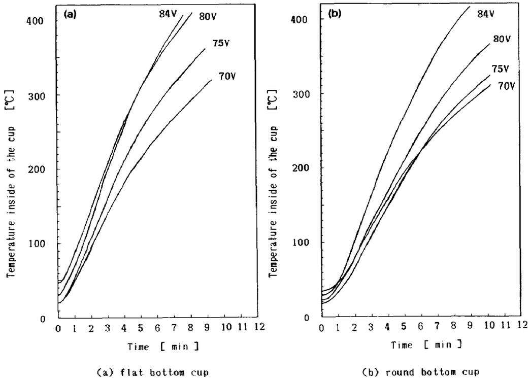
Fig. 4. Heating rate curves of US pressure vessel: (a) flat bottom cup, and (b) round bottom cup. Voltage was varied to 70, 75, 80 and 84 V, respectively.
