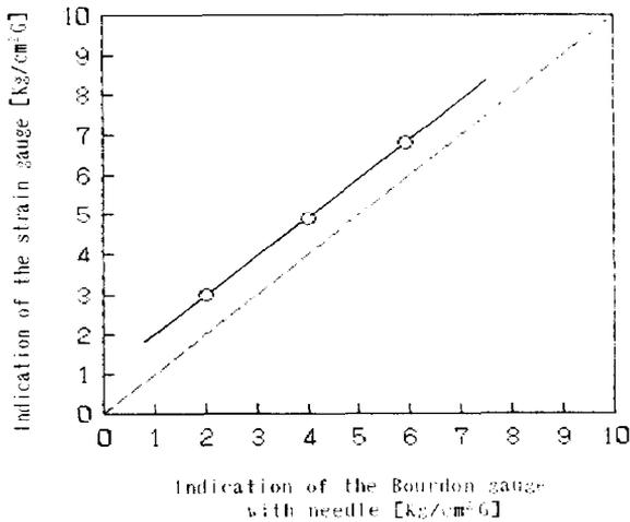
Fig. 10. Maximum pressure measurement: strain gauge vs. Bourdon gauge. Needle effect.
